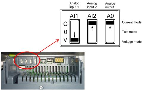
If you're using DVG500 be sure that the corresponding DIP SWITCHES (Al2 for connection on clamps 4-5) is set on CURRENT (C)
