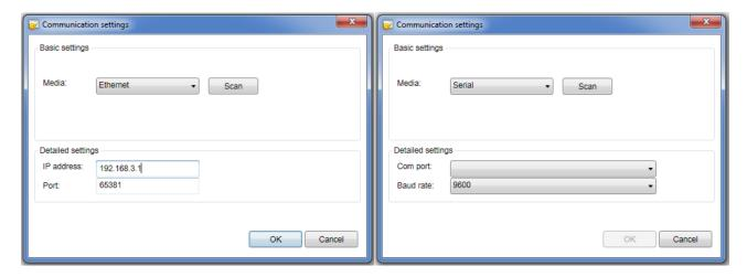
Once the connection parameters are set, click **OK** to search for iDRIVE100 connected to the PC. When the frequency controller is found, its informations appears. You can connect to it by choosing the device's row and clicking **Connect to Selected**.
