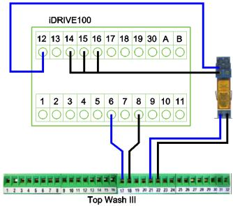
In case you need to keep only one auxiliary pump constantly powered in washing mode, we suggest to put a manual switch on these 2 circuits in order to periodically rotate the auxiliary pump which is constantly powered during washing.
