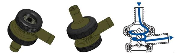
Evolution of the ITP205 model (normally open and equipped with a stainless steel shutter requiring manual locking during washing), the new ITP208 is normally closed and lighter thanks to its main diaphragm capable of automatically opening the internal plastic shutter as required, regardless of milking or washing, reducing the farmer's manual labour.
